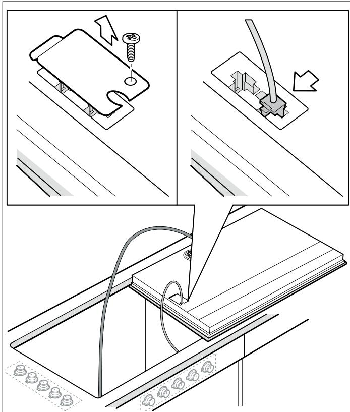
2. The appliance must be secured from below using the hold-down brackets provided, so it does not slip. Position the appliance so that the screws provided are seated loosely in the holes.
