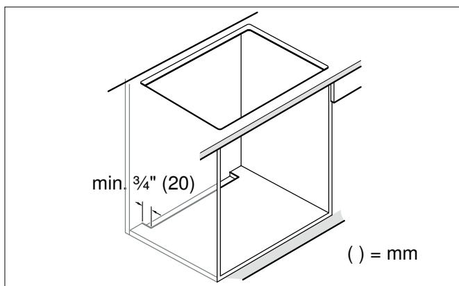
**Note:** If the appliance is installed in an island unit or another installation that is not described here, you must ensure that the cooktop is sufficiently ventilated.
