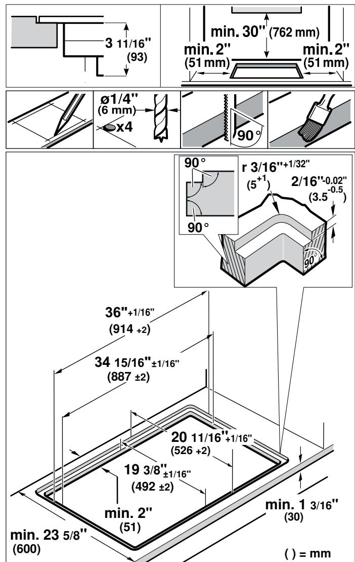
**Flush installation:** The appliance can be installed in the following temperature- and water-resistant countertops:
