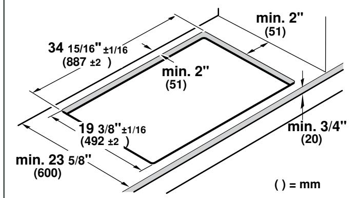
**Flush mounting:** Flush mounting into a countertop is possible.
