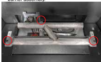
Diagram 2: Slide burner assembly to the right—then remove.
