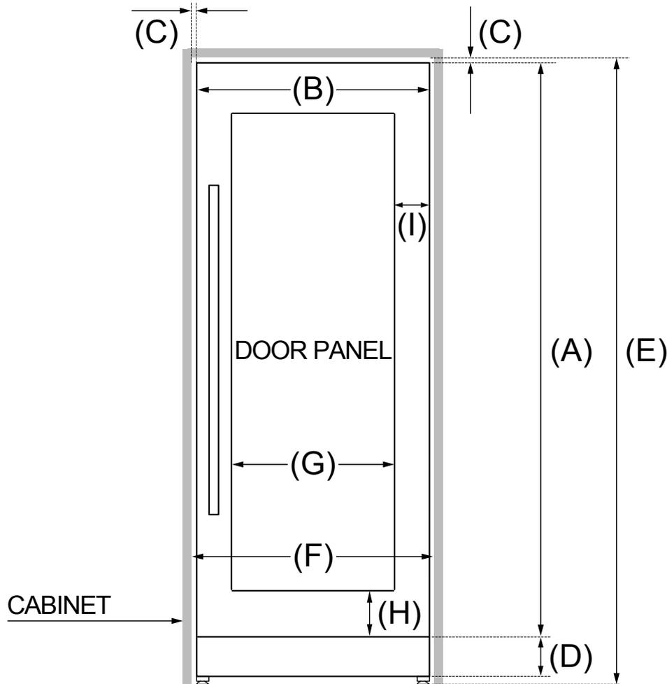
NOTE: The wine column comes with a 4" (100 mm) stainless steel toe kick installed to fit a standard 84" (2134 mm) tall cabinet niche.
