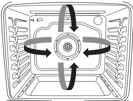
During convection baking or roasting, the bake, broil, and convection elements cycle on and off in intervals while the fan circulates the hot air. During convection broiling, the broil and convection elements cycle on and off.
