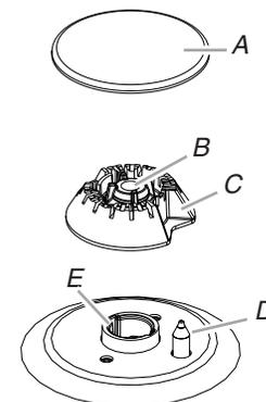
A. Burner cap      D. Igniter electrode
