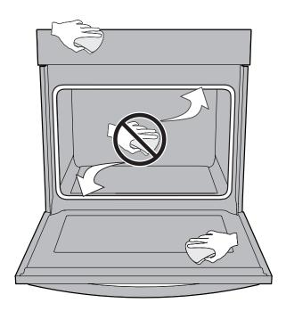
Figure 25: Do not clean oven door gasket
