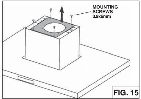
2. Install the external blower plate and secure using (4) 3.9x6 mm screws (Fig.16)
