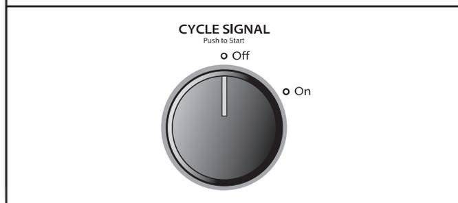
Push and hold the PUSH TO START knob to begin the cycle. Promptly remove garments after cycle has completed to reduce wrinkling. Use the Wrinkle Shield™ feature to avoid wrinkling when you are unable to remove a load from the dryer as soon as it stops.
