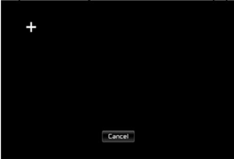
Tap center of the
