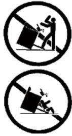
The chains shipped with the range must be properly secured to the rear wall. The height of the bracket from the floor must be determined after the range legs have been adjusted to the desired height and after the range has been leveled. If the chain length is too short to properly secure the range to the rear wall, ask the installer to lengthen it.
