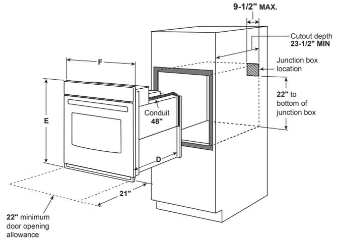
**Electric wall ovens are not approved for installation with a plug and receptacle. They must be hard wired in accordance with installation instructions.**
