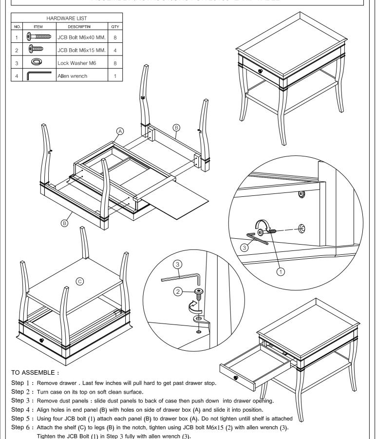
Step 7: Install Dust Panel through drawer opening. Slide Dust panel into slot in backrail then Forward into slot in Front rail.
