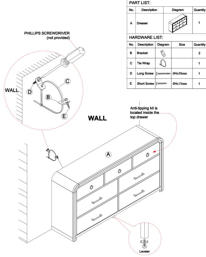
The tipping restraint must be attached at back of Dresser, above and on the right or left.
