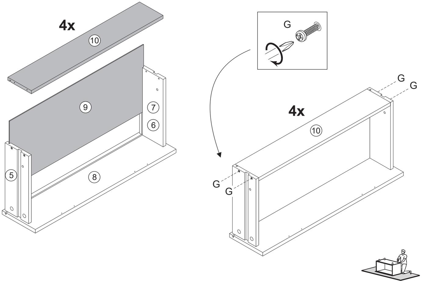
Insert parts 9 and 10 between parts 5, 6 and 7.
