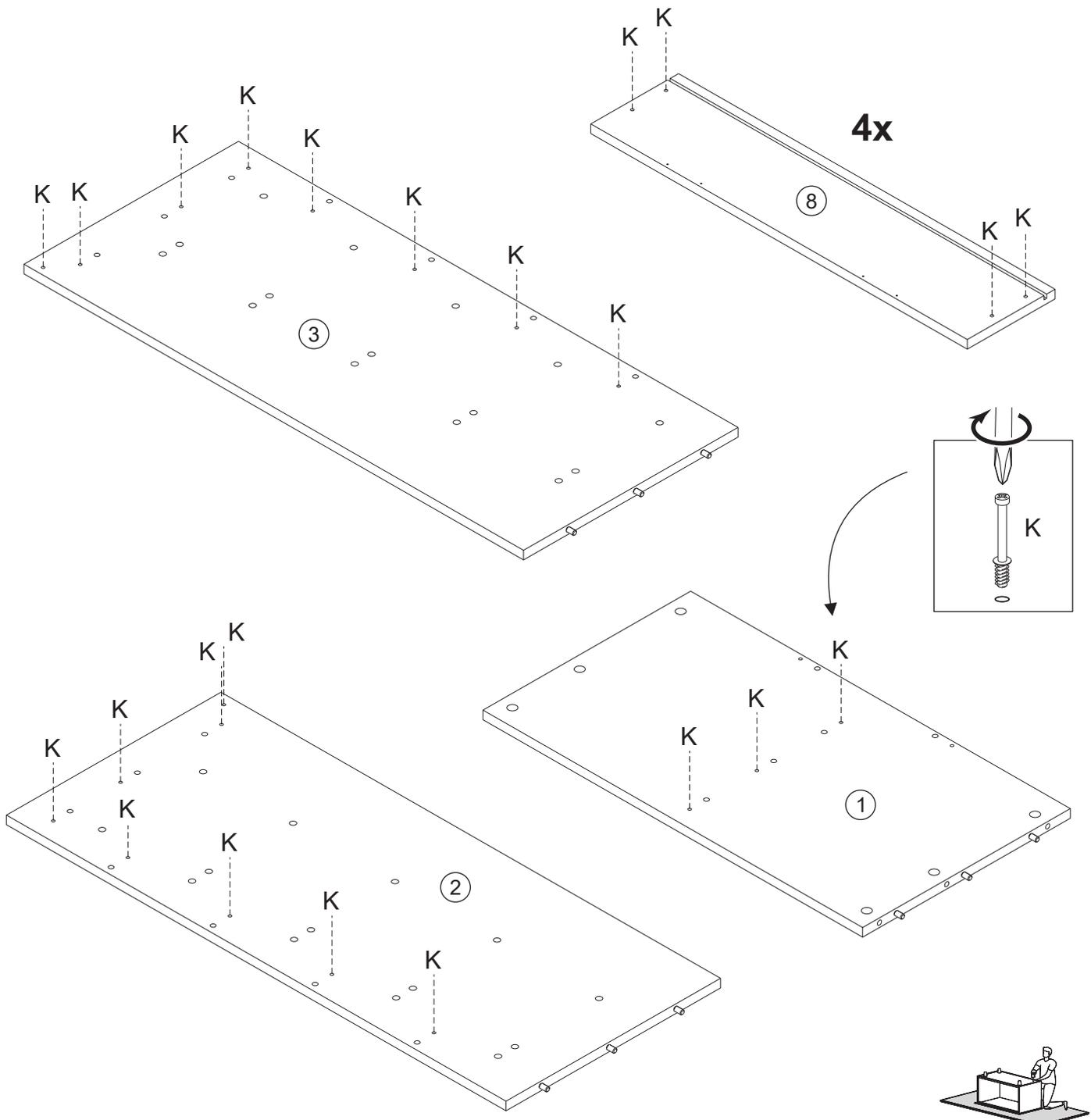
Screw cam bolts (K) into parts 1, 2, 3 and 8 with a phillips screwdriver.
