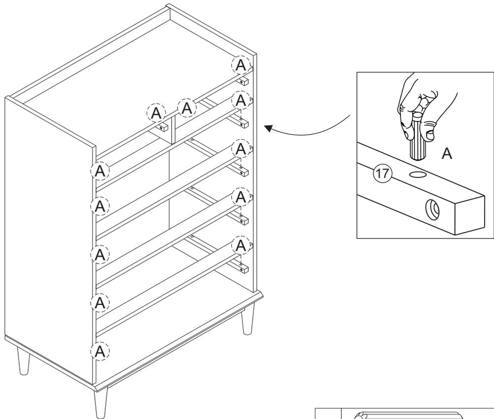
Insert wood dowel (A) into part 17 to be the stop of the drawer.
