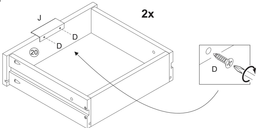
Secure handle (J) with screw (D) and phillips screwdriver, in the pre-drilled holes on the drawer front 20.
