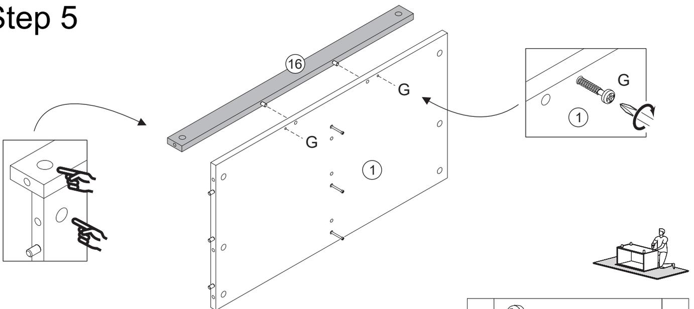
Secure part 16 to part 1 with screw (G) and phillips screwdriver.
