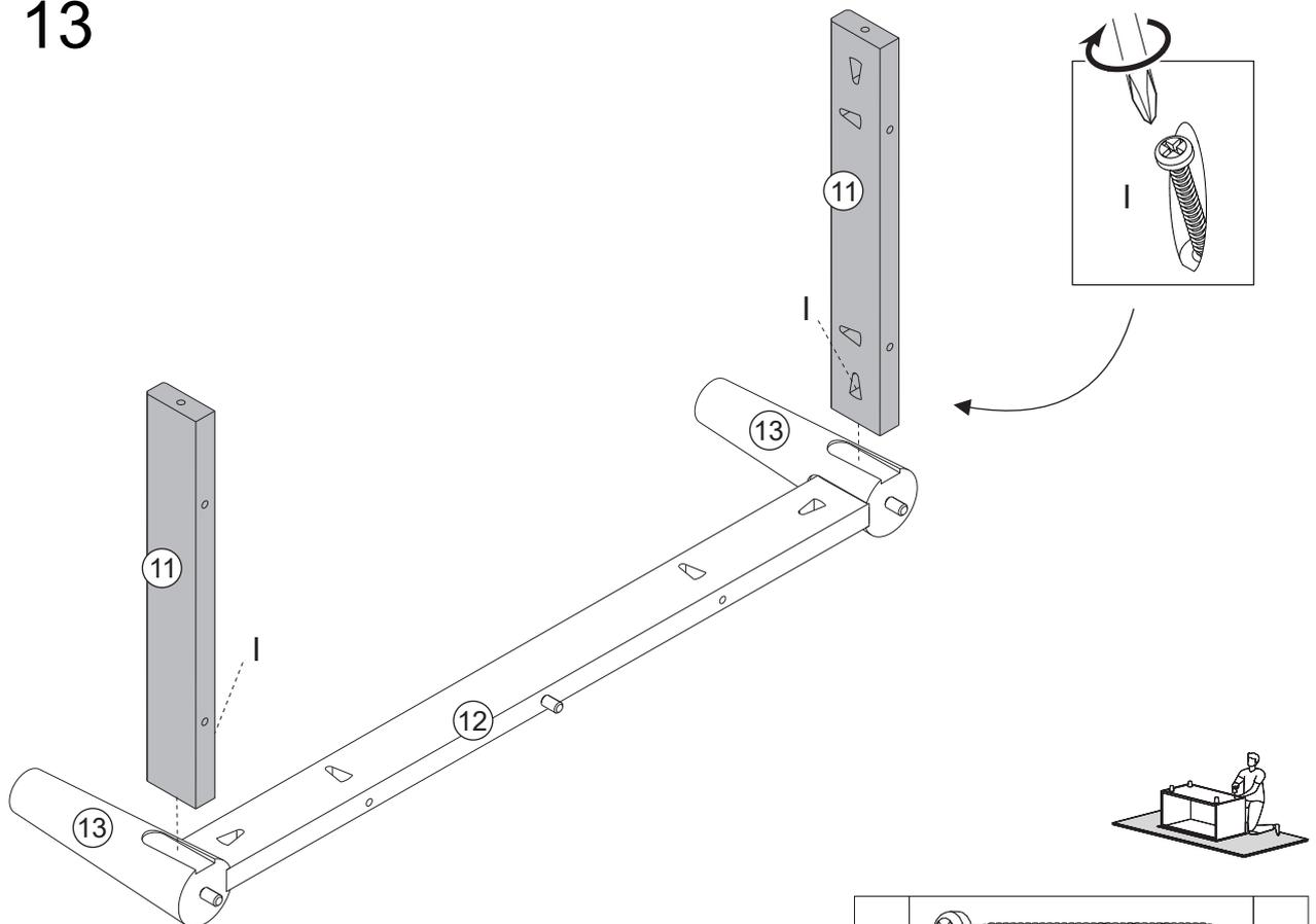
Secure part 11 to parts 13, with screw (I) and phillips screwdriver.
