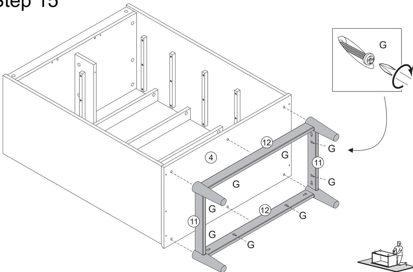
Secure parts 11 and 12 to part 4 with screw (G) and phillips screwdriver.
