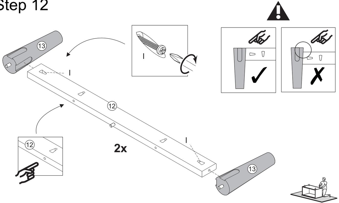
Secure part 12 to parts 13, with screw (I) and phillips screwdriver.
