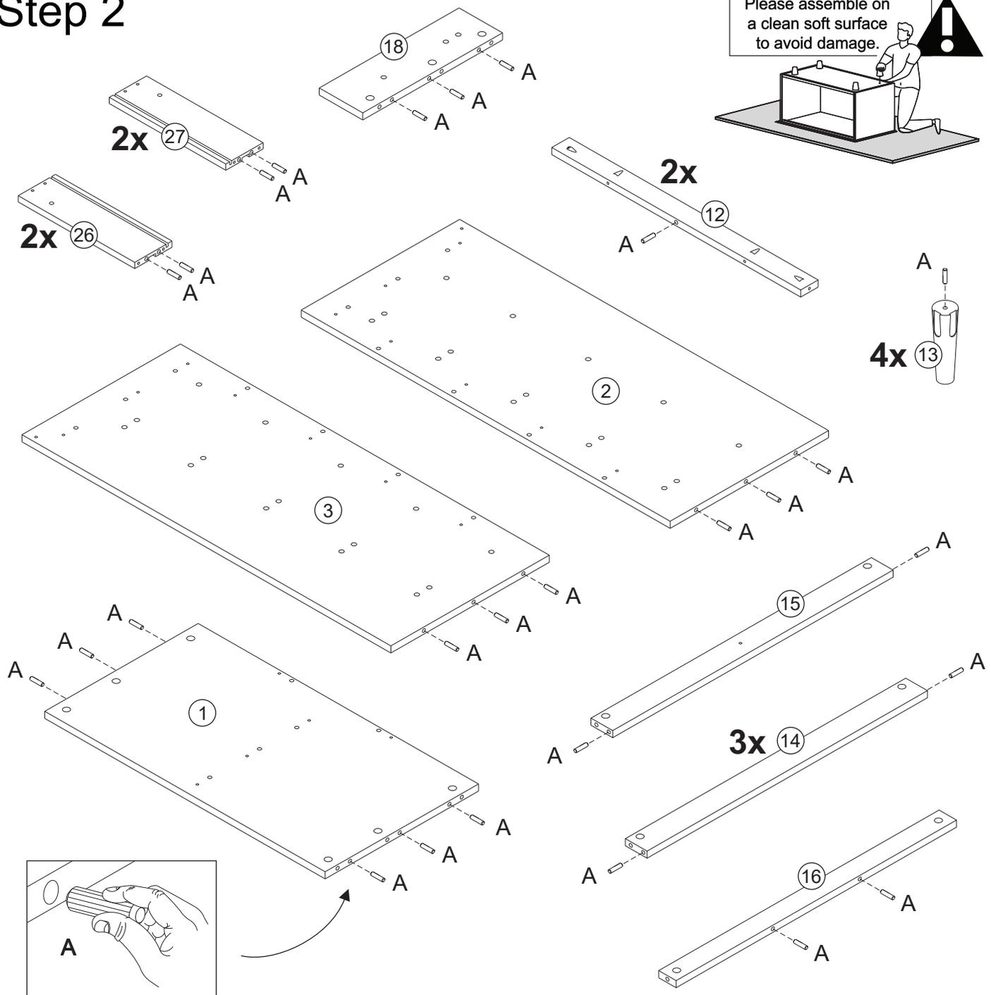
Insert wood dowel (A) into parts
