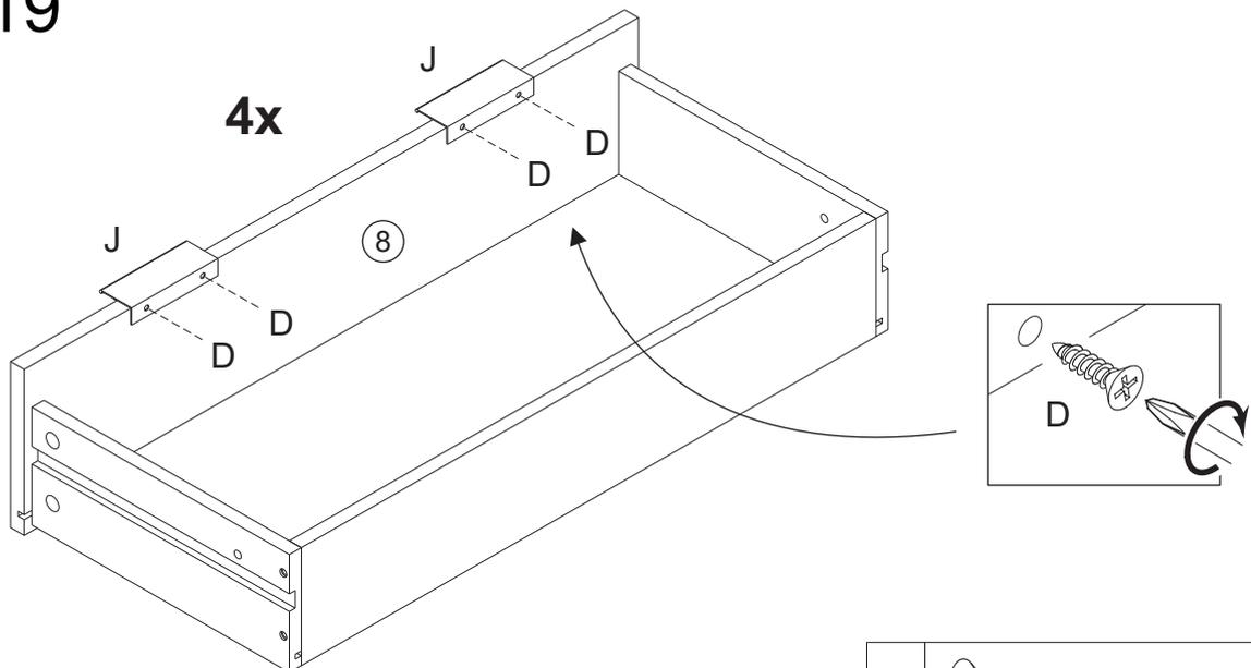
Secure handle (J) with screw (D) and phillips screwdriver,
