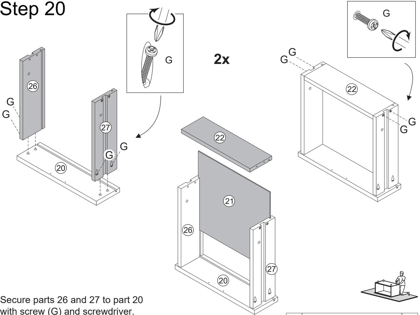
Secure parts 26 and 27 to part 20 with screw (G) and screwdriver.
