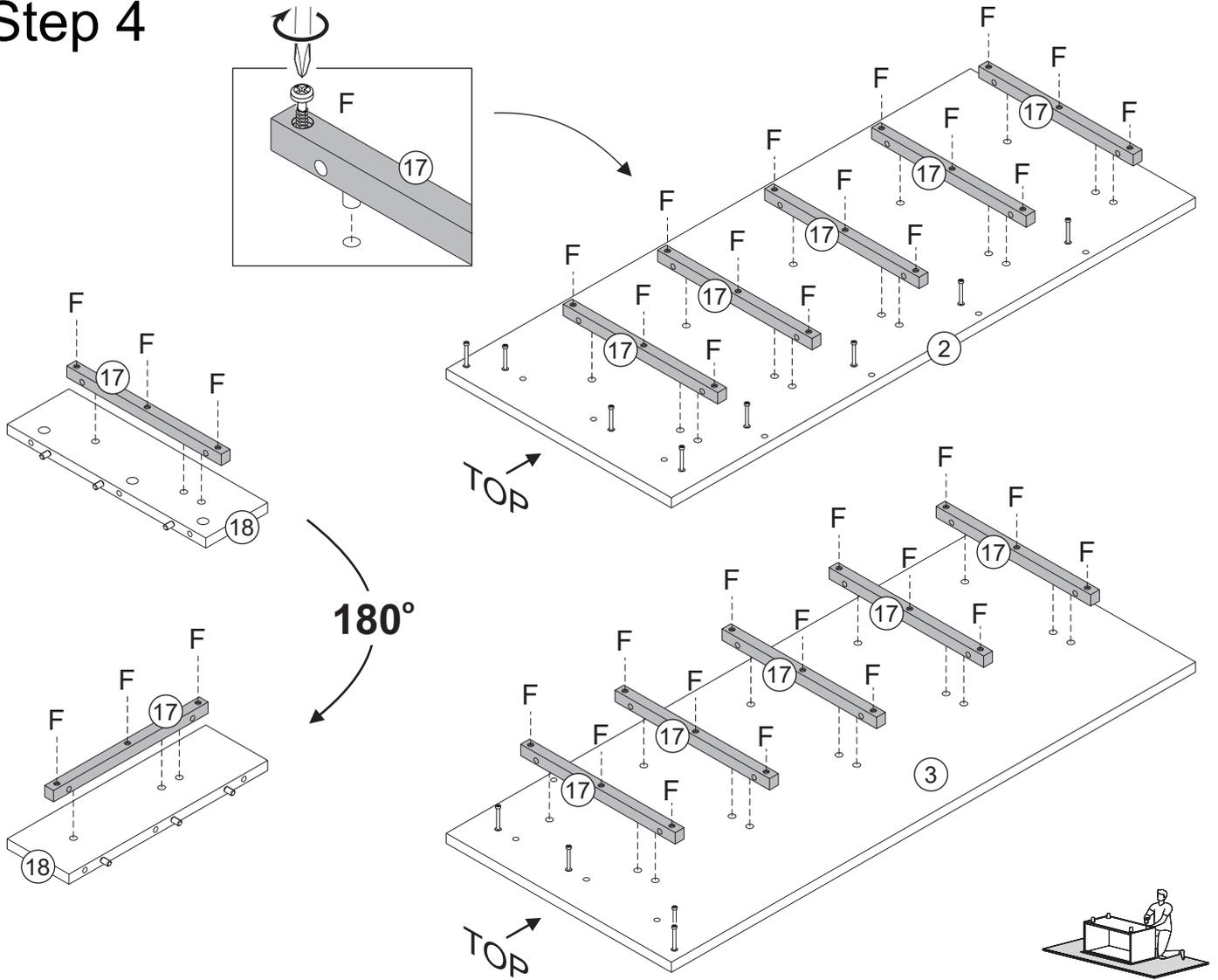
Secure parts 17 to parts 2, 3 and 18 with screw (F) and phillips screwdriver.
