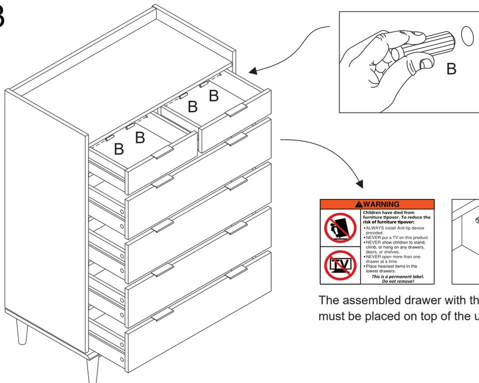
Insert wood dowel (B) on the inside of all drawers, with the drawer inside the unit, after having passed the wood dowel that is in the drawer slide.
