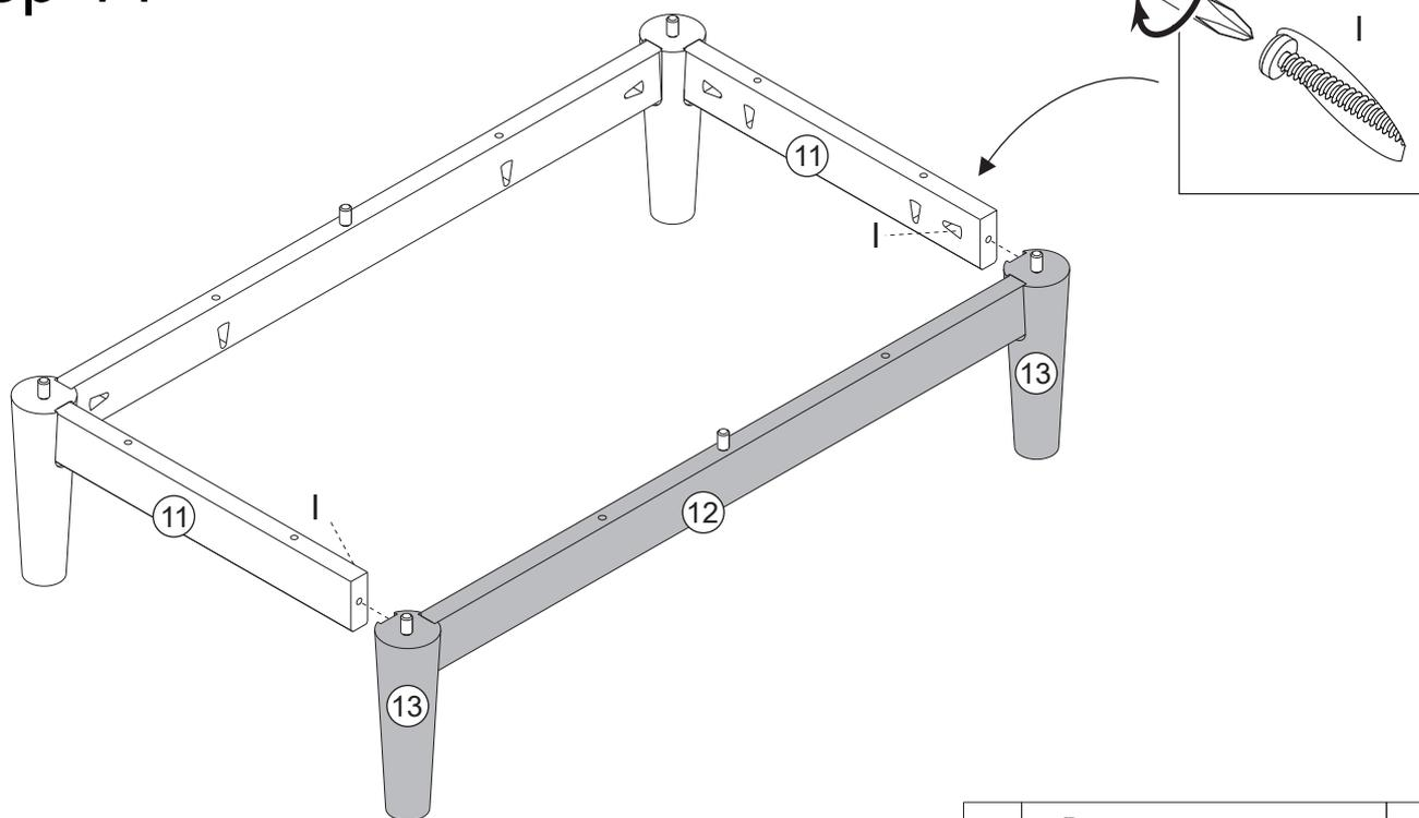
Secure part 11 to parts 13, with screw (I) and phillips screwdriver.
