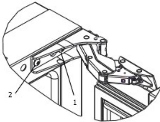
3. Once door is removed, using a Philips Screwdriver remove screws from magnet actuator located on inside and bottom of door. (On Integrated Models magnet actuator will be located on bottom of door.)
