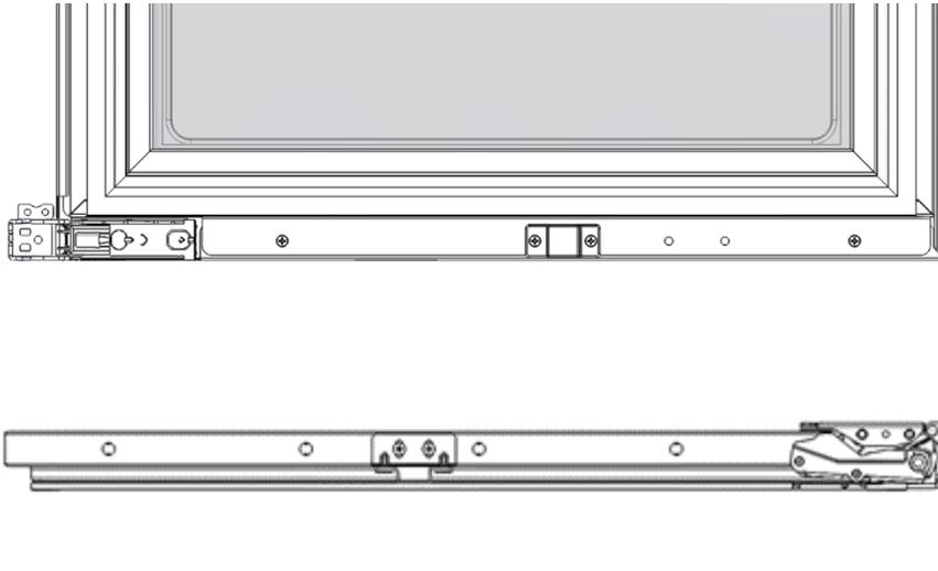
4. Remove caps from top of door. Using a Philips Screwdriver, install magnet actuator on opposite side. Install caps into opposite side.
