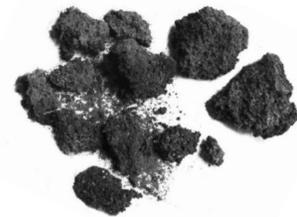
*Above is an example of a pellet “clinker”. This mass of impurities can reduce airflow through the burn pot and create an unsafe burning condition.*
