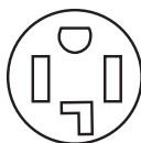
4-wire receptacle (14-30R)
