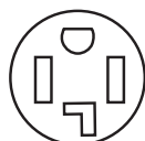
4-Wire Receptacle (14-30R)
