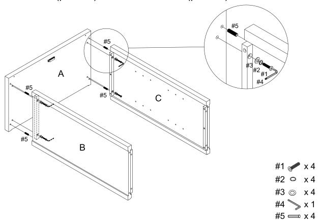
Step 4. Attach bottom panel (part D) to panels (parts B & C) using wood dowels (part #5), bolts (part #1), spring washers (part #2), flat washers (part #3) and allen wrench (part #4).
