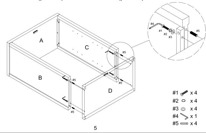
Step 5. Attach legs (parts H & I) to bottom panel (part D) using wood dowels (part #5), bolts (part #1), spring washers (part #2), flat washers (part #3) and allen wrench (part #4).
