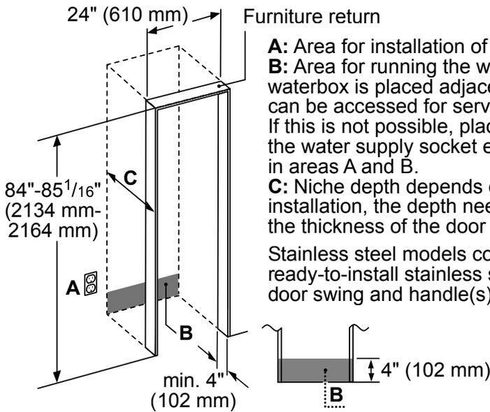
**A:** Area for installation of power connection.
