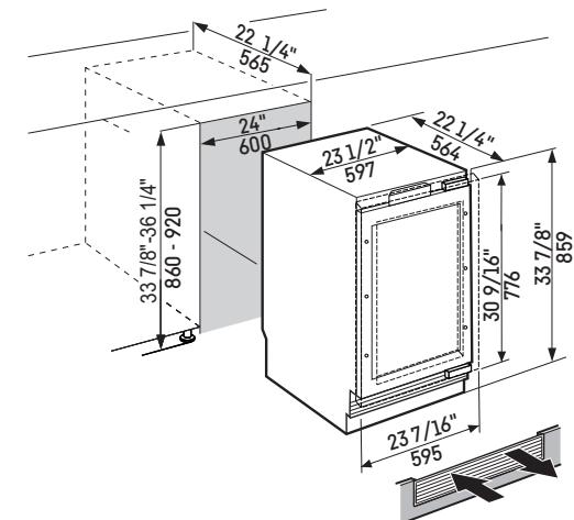
This is a fully integrated undercounter model which means that it is fully enclosed by a kitchen cabinet. This type of cabinet must be carefully constructed using the correct dimensions and it must provide suitable ventilation to ensure proper appliance operation. The floor on which the appliance stands must be horizontal, and level and the kitchen cabinets must be aligned horizontally and vertically.
