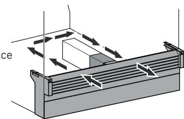
After installing the kitchen cabinet door, there must be a ventilation gap between the appliance ventilation grille and the kitchen cabinet door. The ventilation grille is movable to guarantee sufficient ventilation.
