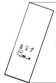
Do not install this unit next to any other refrigerator, freezer or wine column except another Liebherr model. Liebherr models are designed to allow for Side-by-Side installation. They are equipped with a heating system to eliminate condensation when units are installed Side-by-Side. Installing this unit next to any other refrigerator, freezer or wine column can cause condensation or cause damage to the Liebherr unit.
