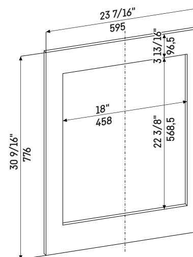
The door should be at least 5/8 in. (16 mm) thick to allow the connecting rails to be fastened to it. The maximum thickness of the door panel is 3/4 in. (19mm).
