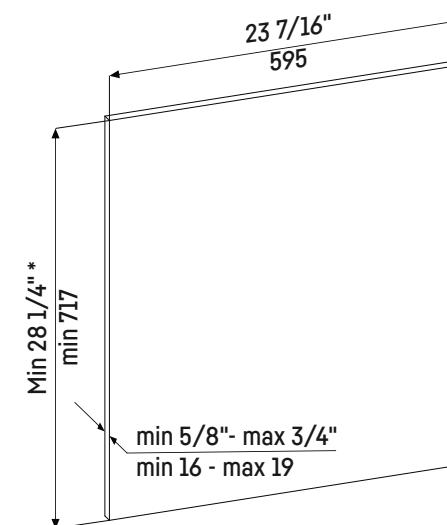
Custom panels should be at least 5/8"(16mm) and a maximum of 3/4"(19mm) thick.
