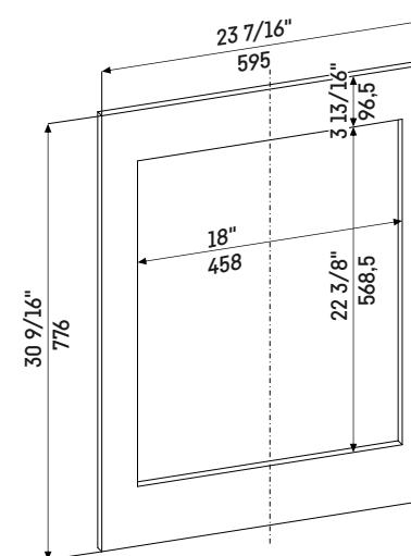
The door should be at least 5/8 in. (16 mm) thick to allow the connecting rails to be fastened to it. The maximum thickness of the door panel can be 3/4 in. (19mm).
