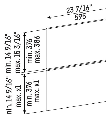
Custom panels should be at least 5/8"(16mm) and a maximum of 3/4"(19mm) thick. Maximum value must not exceed the maximum ventilation cross-section of 24 in² (150 cm²).
