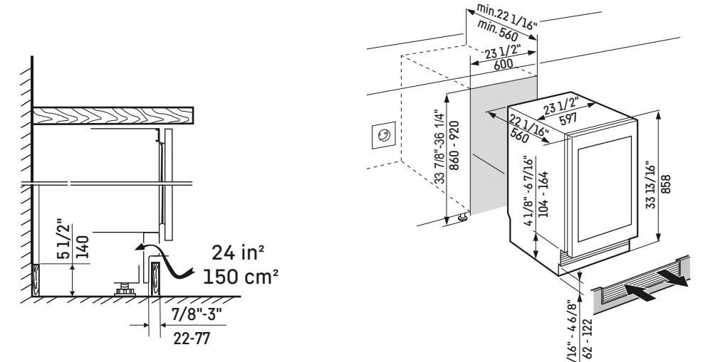
This is a fully integrated undercounter model which means that it is fully enclosed by a kitchen cabinet. This type of cabinet must be carefully constructed using the correct dimensions and it must provide suitable ventilation to ensure proper appliance operation. The floor on which the appliance stands must be horizontal, and level and the kitchen cabinets must be aligned horizontally and vertically.
