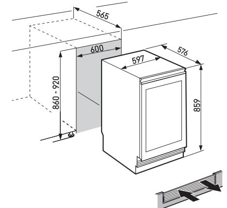
This is a built-in undercounter model which means that it is enclosed by a kitchen cabinet. This type of cabinet must be carefully constructed using the correct dimensions and it must provide suitable ventilation to ensure proper appliance operation. The floor on which the appliance stands must be horizontal, and level and the kitchen cabinets must be aligned horizontally and vertically.
