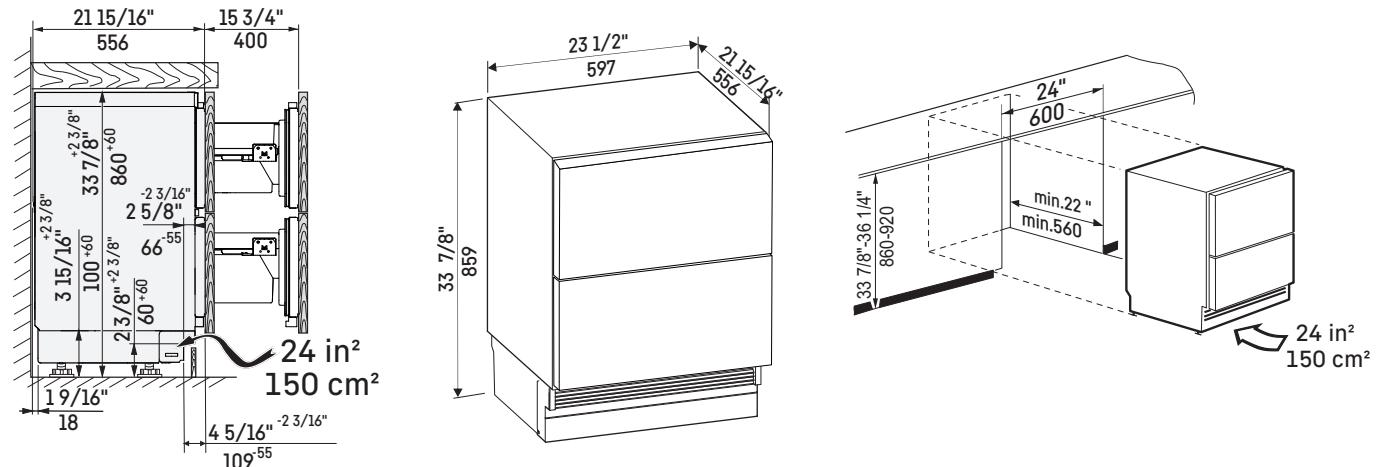
This is a fully integrated undercounter model which means that it is fully enclosed by a kitchen cabinet. This type of cabinet must be carefully constructed using the correct dimensions and it must provide suitable ventilation to ensure proper appliance operation. The floor on which the appliance stands must be horizontal, and level and the kitchen cabinets must be aligned horizontally and vertically.
