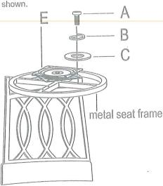
2)Attach swivel plate(E) to metal base by using 4pcs Philip head bolts(A),4pcs Lock washers(B) and 4pcs flat
