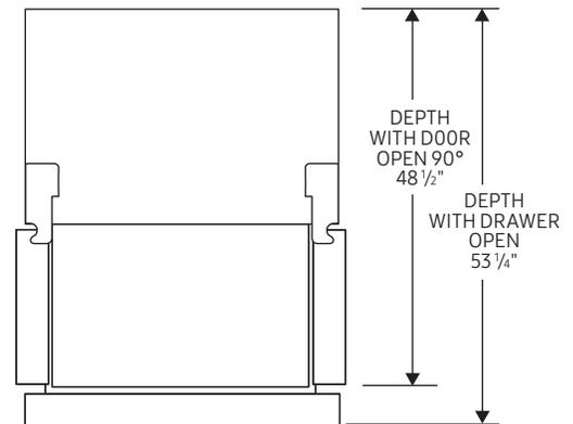
TOP OF REFRIGERATOR WITH DOORS OPEN  $125^\circ$
