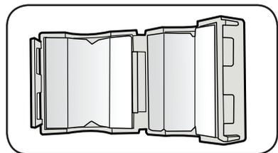
Lift up to release the lock and open the core.
