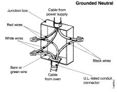
Refer to Figure A, where local codes allow the connection of GROUND wire from the oven to the branch circuit NEUTRAL wire (gray or white colored wire):
