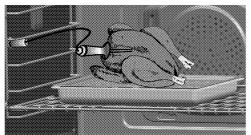
The probe is used to measure the central temperature of meats and poultry such as chicken or turkey by sticking the thin and long part into the meat and attaching the other end to its slot on the side wall of the chassis.
