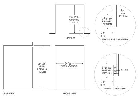
NOTE: 3<sup>1</sup>/2" (89) finished returns will be visible and should be finished to match cabinetry.
