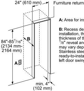
A: Area for installation of power connection.
