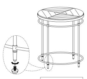
Adjust leveler if needed to level case on uneven floor
