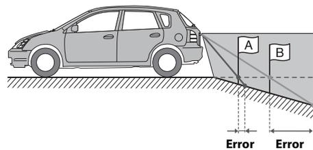
In the case of a downward slope behind the car, the distance guides are displayed farther from the rear bumper than the actual distance. If there is an obstacle on the downward slope, it seems closer than its actual position. Also, an error may occur between the guidance and the actual path of the car on the road surface.
