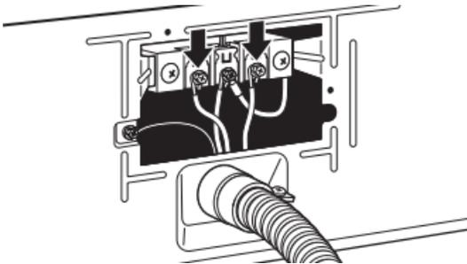
Place hooked ends of remaining direct wire cable wires under outer terminal block screws (hooks facing right). Squeeze hooked ends together and tighten screws. Insert tab of terminal block cover into slot of dryer rear panel. Secure cover with hold-down screw. Now, go to "Venting Requirements."
