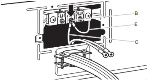
Connect neutral bond wire (E) and neutral wire (white or center wire) (C) of power supply cord or cable under center terminal block screw (B). Tighten screw.
