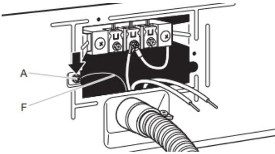
Connect ground wire (green or bare) (F) of direct wire cable under green external ground conductor screw (A). Tighten screw.
