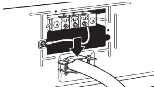
Put power supply cord through the strain relief. Be sure that the wire insulation on the power supply cord is inside the strain relief. The strain relief should have a tight fit with the dryer cabinet and be in a horizontal position. Tighten the strain relief against the power supply cord. Do not overtighten the strain relief screws.
