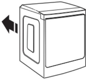
Move dryer to final location. Avoid crushing or kinking the vent. After dryer is in place, remove corner posts and cardboard from under dryer.
