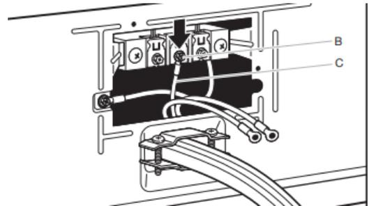
Connect neutral wire (white or center) (C) of power supply cord under center terminal block screw (B). Tighten screw.
