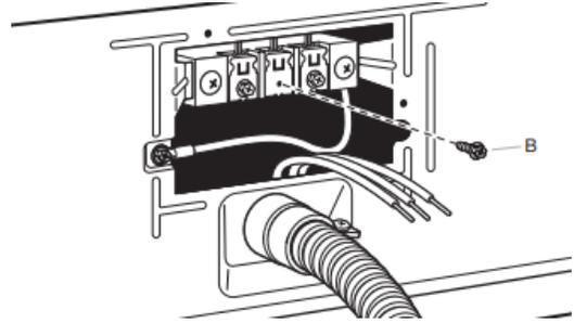
Remove center terminal block screw (B).
