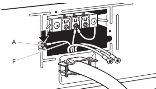
Connect ground wire (F) (green or bare) of power supply cord under green external ground conductor screw (A). Tighten screw.
