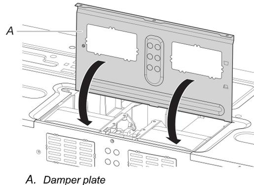
8. Secure damper plate with 2 screws removed in Step 1.
