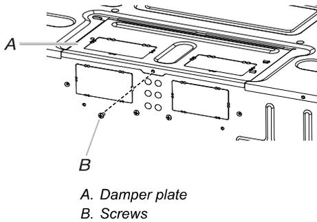
2. Turn and hold the damper plate vertically as shown.
