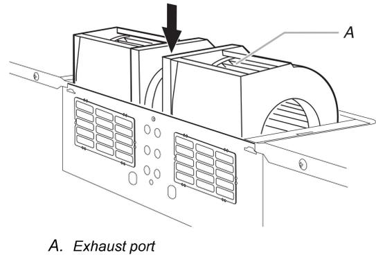
**IMPORTANT:** If blower motor is not positioned with flat side facing the back of the microwave oven (as shown), performance will be poor.
