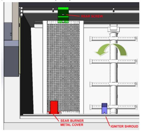
2. With the burner removed, you will see 2 threaded holes on either side of the igniter. Mount the new shroud as shown below with the screws provided, but leave the screws loose temporarily.
