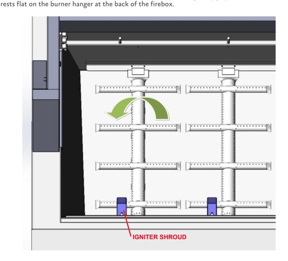
2. Adjust the shroud down onto the burner so it hugs the cross tube / channel as close as possible, but not so far that the burner will not lay flat on the burner hanger at the back of the firebox. Tighten the screws on either side of the shroud.
