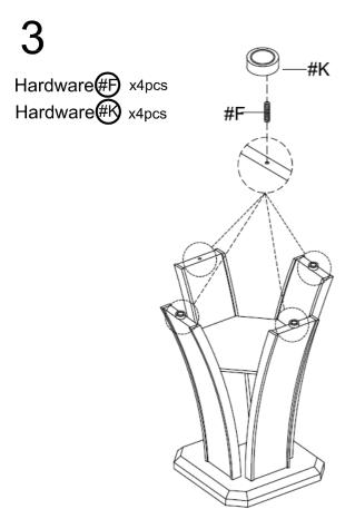
Insert the 4 threaded studs (#F) into the top of the stands (#3). Then insert the 4 spacers (#K) onto the 4 threaded studs (#F).
