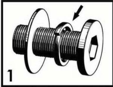
1 When lock or spring washer is used in an assembly, please make sure the lock or spring washer is placed between the larger flat washer and the head of the screw or bolt.
