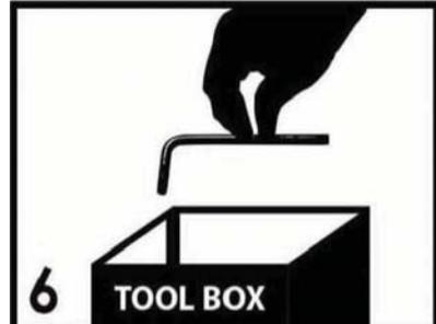
6 Save the instructions and store the Allen wrench or any supplied tool for later maintenance. After two weeks, check and tighten any loose hardware and repeat again every six months thereafter.
