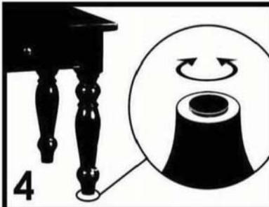
4 Some furniture comes with height adjustment knobs underneath each leg. To lower or to raise each leg, you need to turn clockwise or counterclockwise, respectively.
