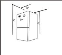
This refrigerator needs to be installed independently and cannot be used as a built-in. Otherwise, it will cause problems such as failure to install into the cabinet, the performance and life of the product are reduced. And the manufacturer does not provide basic product warranty.
