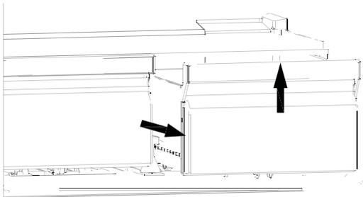
2. The roller seat is stuck in the box tank groove, press the arrow in the direction of the image, remove the roller seat, clean the box tank groove as needed.
