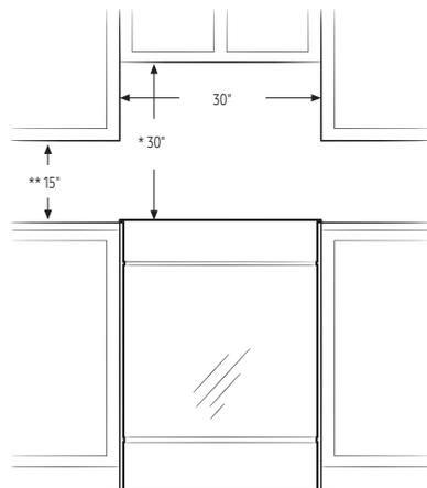
\* 30" minimum clearance between the top of the cooking surface and the bottom of an unprotected wood or metal cabinet; or 24" minimum when the bottom of the wood or metal cabinet is protected by not less than 1/4" of flame retardant millboard covered with not less than no.28 MSG sheet steel, 0.015" stainless steel, 0.024" aluminum, or 0.020" copper.
