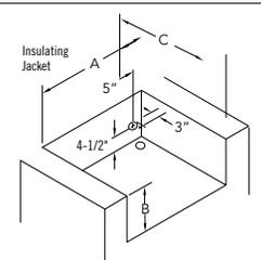
**Note:** Insulating jacket required for all grills installed into a combustible enclosure. For natural gas grills, Lynx recommends using 3/4" gas lines. Side burners may be rotated 90 degrees. See installation manuals for details.
