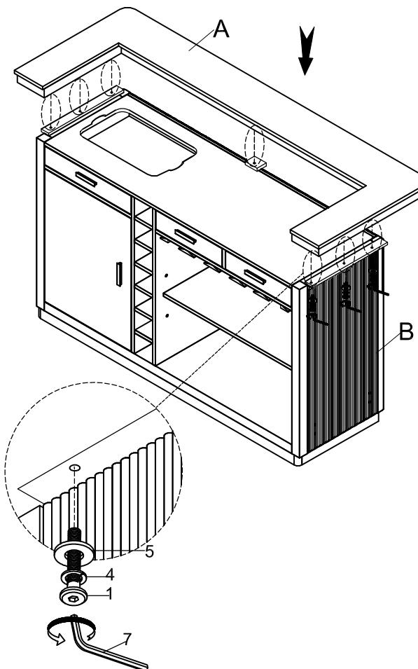
STEP 2 : Attach the side foot rest at both the sides.
