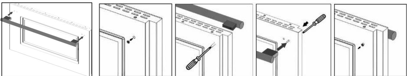
1. Remove the black rubber cap on the inside of oven door. (Do not throw it away).
