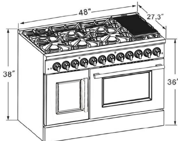
This range may be installed directly adjacent to existing countertop-height cabinets (36" or 91.5 cm from the floor). To achieve the best look, the cooktop should be level with the cabinet countertop. This can be accomplished by raising the unit using the adjustment spindles on the legs.
