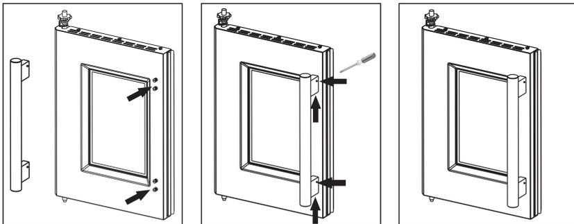
1. Align the handle with the screw on the door.
