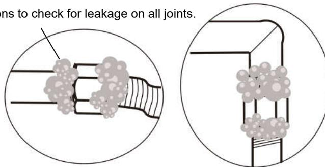
**⚠WARNING** DO NOT use a flame to check for gas leakage.
