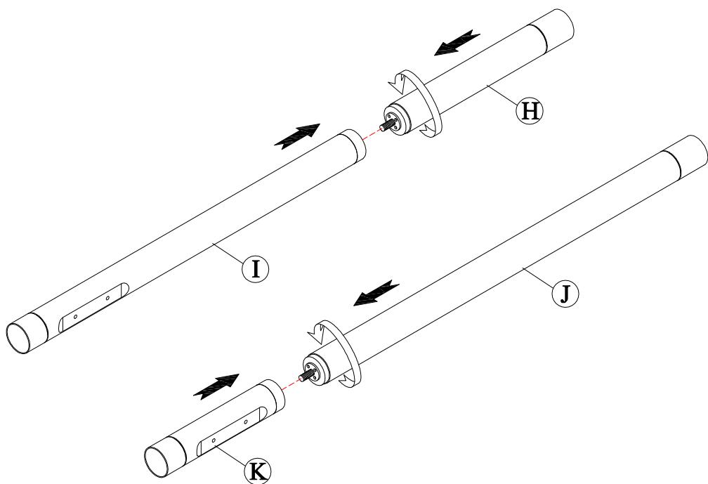
Attach the parts of the Headboard Leg (H,I) and Footboard Leg (J,K) by turning as clockwise direction.
