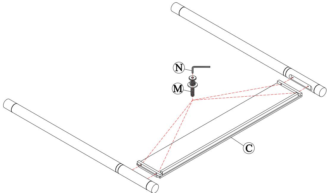
Attach Footboard Leg (L&R) to Footboard (C) by using Bolt (M) and tighten with Allen Key (N).
