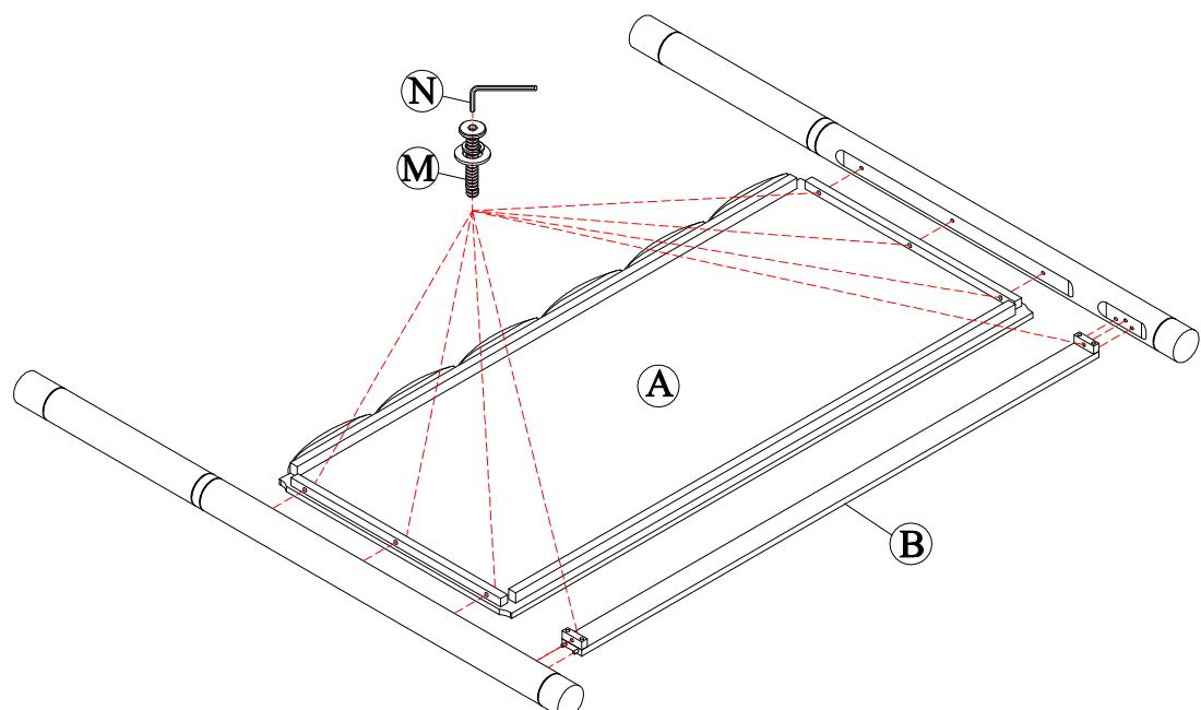
Attach Headboard Leg (L&R) to Headboard (A) and Cross Bar (B) by using Bolt (M) and tighten with Allen Key (N).
