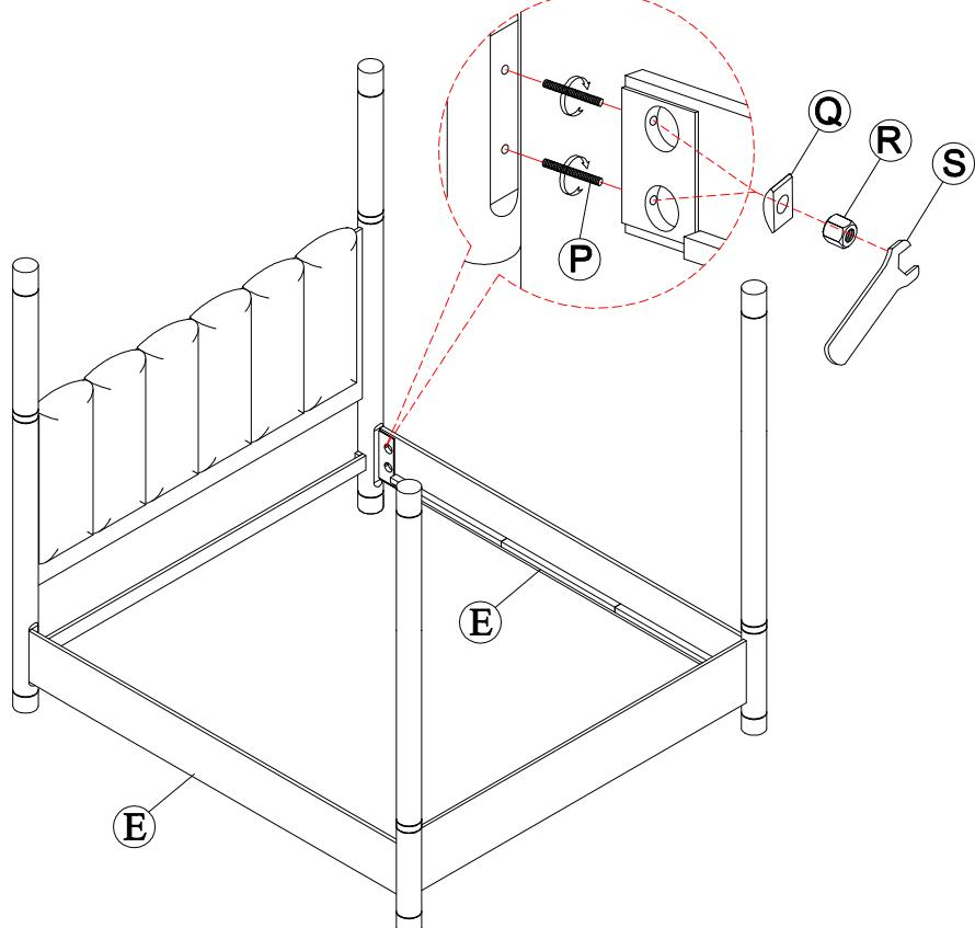
Attach Threaded Rods (P) to the Headboard and Footboard, then align side rail (E) to the Threaded Rods (P). Secure by using Nuts (R) with Half Moon Nut (Q).
