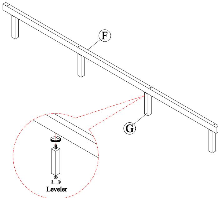
Attach Support Leg (G) to Center Support (F) by turning as clockwise direction.
