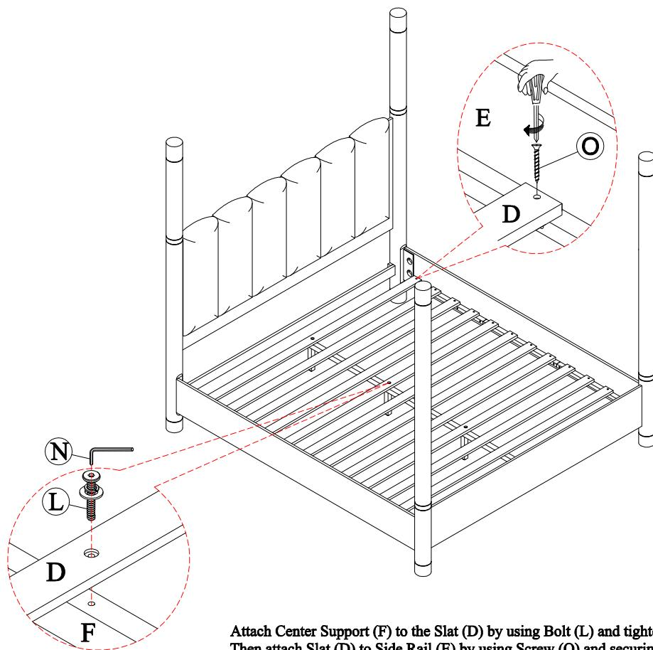
Attach Center Support (F) to the Slat (D) by using Bolt (L) and tighten with Allen Key (N). Then attach Slat (D) to Side Rail (E) by using Screw (O) and securing with Screw - driver (not included).
