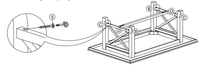
STEP 5 To level the table, turn the table right side up and tighten the bolts with Allen key (6).
