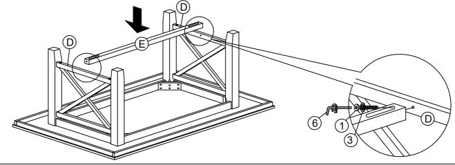
STEP 4 Assemble the leg bases by using a screwdriver with hardware 5.
