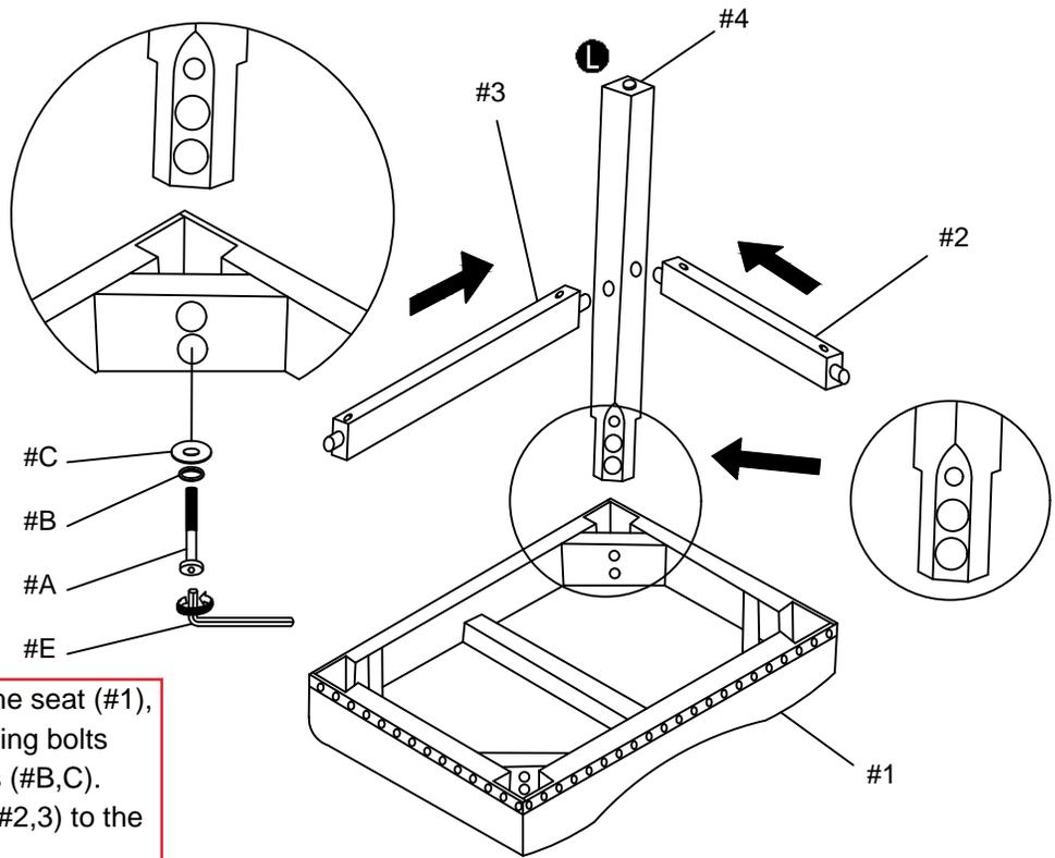
Align leg (#4) to the seat (#1), then secure by using bolts (#A) with washers (#B,C). Insert stretchers (#2,3) to the leg (#4).
