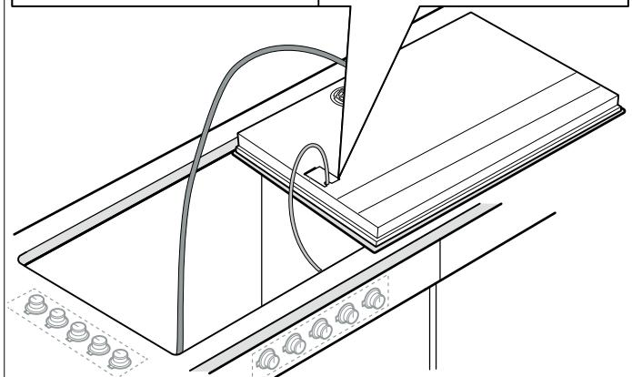
2. The appliance must be secured from below using the hold-down brackets provided, so it does not slip. Position the appliance so that the screws provided are seated loosely in the holes.
