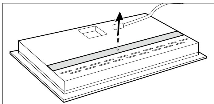
The heat shield will be able to rotate freely, as shown in the illustration.
