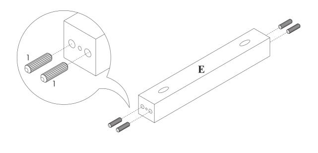
STEP 2: Attach Lower Rail (D) to Rail between Foot (E) with screws (2) and a Phillips head screw driver (not provided).
