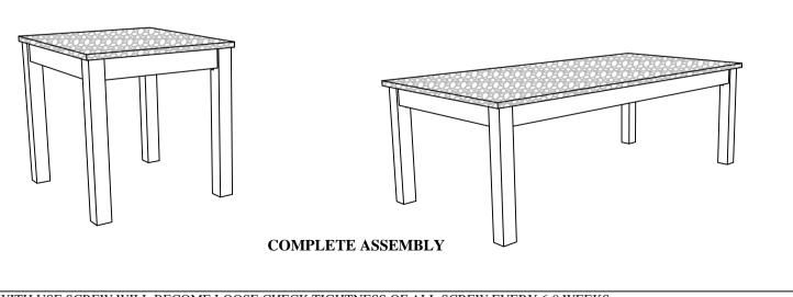
NOTE: MUST TIGHTEN SCREWS PERIODCALLY WITH USE SCREW WILL BECOME LOOSE CHECK TIGHTNESS OF ALL SCREW EVERY 6-8 WEEKS.
