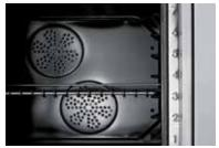
Two large-blade fans positioned on the diagonal axis and subsidiary air vents at the top and bottom of the oven cavity provide balanced airflow and even heat distribution.
