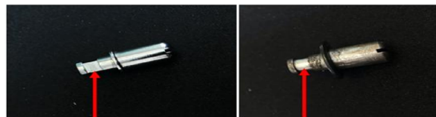
New pin – flat edges where the M6 x 10mm grub screw holds the pin in place
