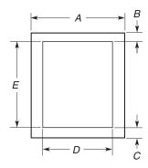
A. 27" (68.6 cm) min. cabinet width on 27" (68.6 cm) models 30" (76.2 cm) min. cabinet width on 30" (76.2 cm) models
