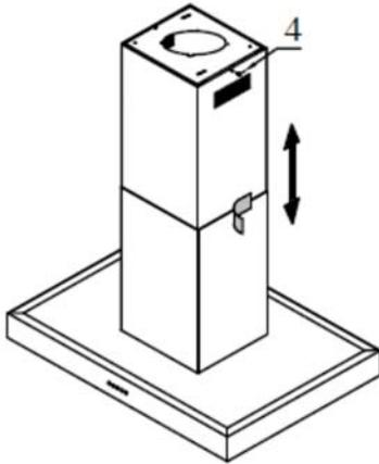
Slide the inner flue upwards slowly & carefully to avoid scratch. Secure the position with two screws onto the ceiling frame.
