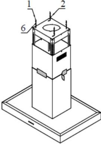
Lift up the hood and mount the ceiling frame to the ceiling ensuring that it is enough to handle the weight of the hood. Connect the power supply and ducting system.
