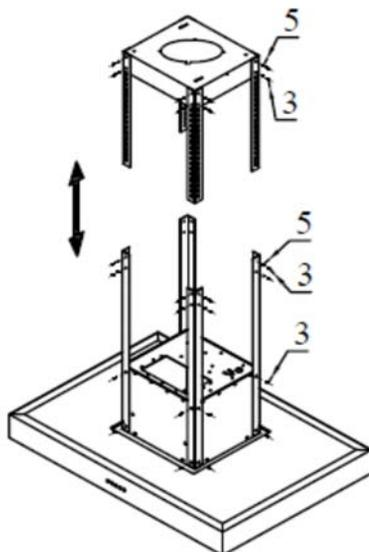
Adjust the brackets to the desired height
