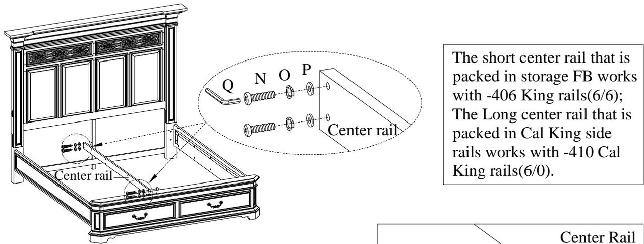
**STEP 7:** Attach 2 support legs (for center rail) to the center rail using 4 bolts(N), lock washers(O) and flat washers(P). Use the Allen Wrench (Q) to tighten all of the bolts.
