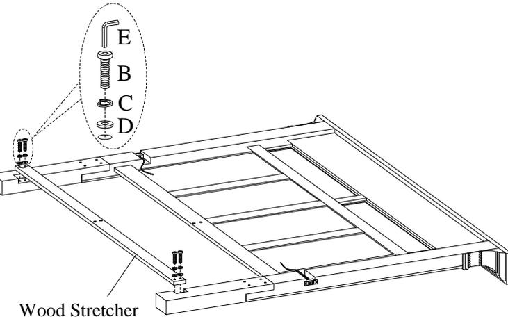
**STEP 2:** Attach the wood stretcher to the legs by using 4 bolts(B), lock washers(C) and flat washers(D).
