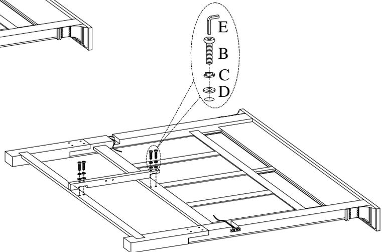
**STEP 3:** Attach the center support leg to headboard and wood stretcher by using 4 bolts(B), lock washers(C) and flat washers(D).
