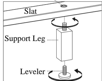
**STEP 6:** Attach the support legs with leveler to the slats. Adjust the levelers on bottom of support legs when necessary.
