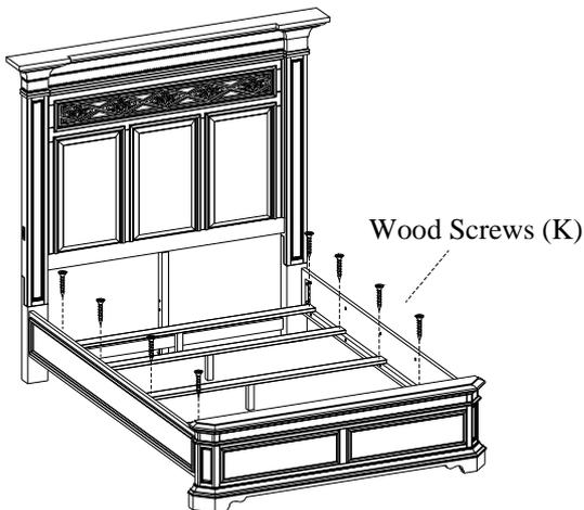
**STEP 7:** Arrange the slats on the slat bearers equally and attach to the slat bearers with wood screws (K).
