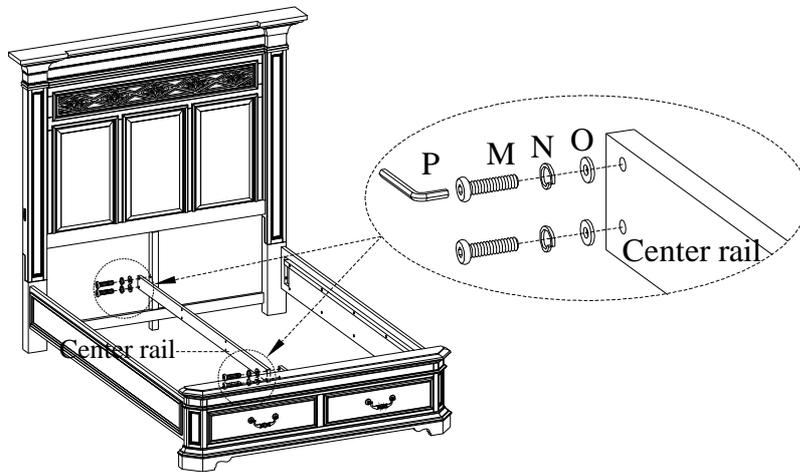
**STEP 7:** Attach 2 support legs (for center rail) to the center rail using 4 bolts(M), lock washers(N) and flat washers(O). Use the Allen Wrench (P) to tighten all of the bolts.
