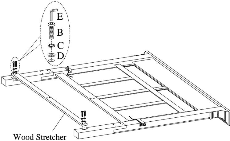
**STEP 2:** Attach the wood stretcher to the legs by using 4 bolts(B), lock washers(C) and flat washers(D).
