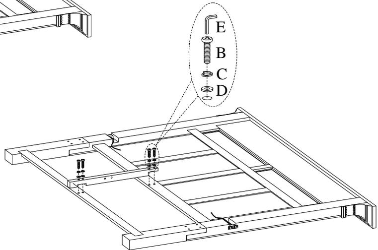
**STEP 4:** Put footboard upside down on a padded, clean surface. Attach support legs (for pedestal) to footboard. Turn footboard right side up.
