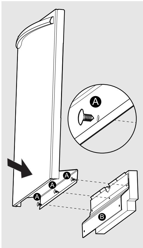
1. Align 3 provided push buttons with barrier (A) holes to corresponding kickplate (B) holes.
